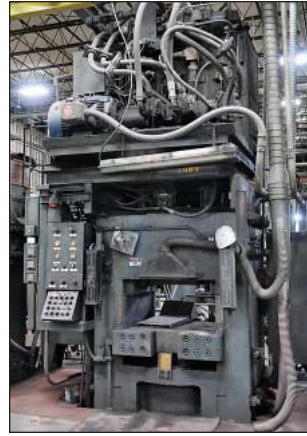
(3) 1,100 Ton Erie No. 1582 Up-Acting Hydraulic Compression Presses
