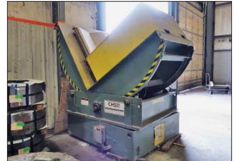
60" x 10,000 Lb. CHS Model PSU-100 Coil Upender
