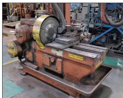
22" Sundstrand Model 12 Automatic Rotary Groover
