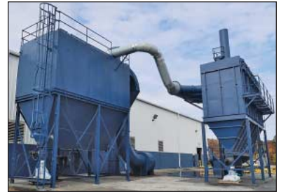
(2) Torit Bag Houses with 100 HP Blower 10,000 CFM
