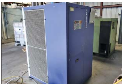
Beko Model DARAx2000NA-RB Air Dryer
