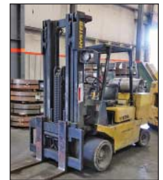
12,000 Lb. Hyster Model S120XLS LP Gas Solid Tire Lift Truck
